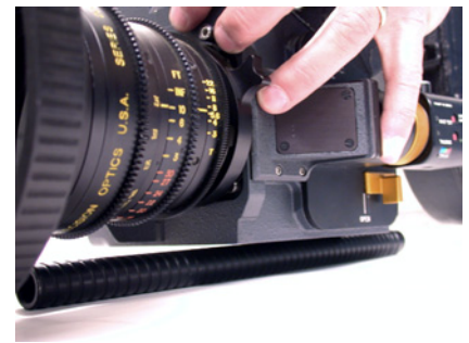
Finding the camera's side to side c.g. To find the vertical c.g., lay the camera on its side.
