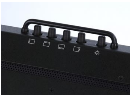
Controls for the FLG built into the monitor. Not all monitors have these framelines installed
