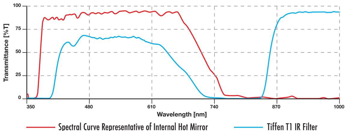
This filter is manufactured using Tiffen’s proprietary ColorCore™ technology, where each effect is captured between two pieces of glass. This allows Tiffen to grind and polish both surfaces providing the cinematographer with perfect parallelism and worry free handling.
